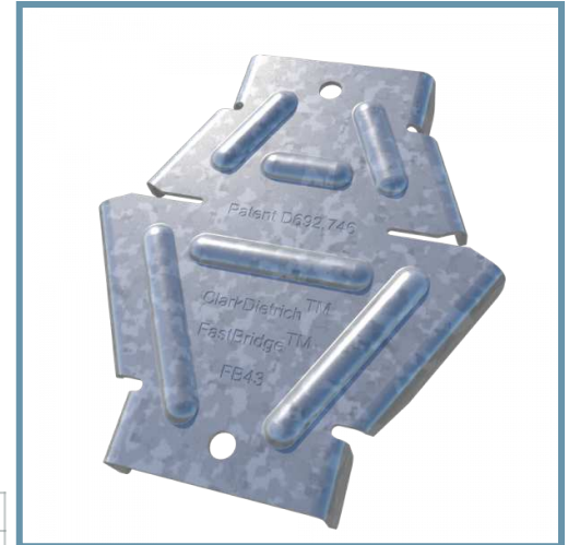
43mils (18ga) light-duty clip for use with 20ga to 16ga structural studs.
